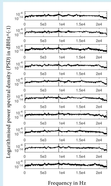
Fig. 8: The peaks of the sound spectra superimpose perfectly with the predicted ground mode frequencies of the open-end neck resonance ground mode (black lines in the spectra). Data was taken from ten different coins. From top to bottom, the coins are: 1 Euro, 0.2 AUD, 0.2 CHF, 1 CHF, 2 CHF, 5 CHF, 2 Euro, 0.1 NZD, 0.5 NZD, 0.2 SGPD.
