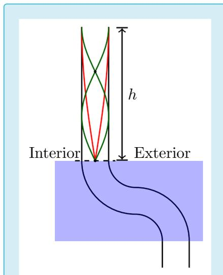
Fig. 1: Open end modes of resonance. The blue area shows the zone in which the curvature of the bottle leads to perturbations of sound waves travelling along the bottle neck and where thus a nodal point is assumed to be. Note that the ground mode  $\lambda_0$  pertains to the red curve, while the first upper mode  $\lambda_1$  pertains to the green curve.
