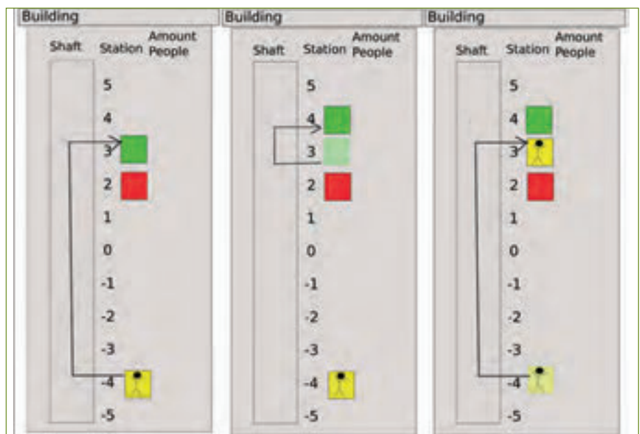
Figure 7: The control-object manages the traffic: The yellow cabin wants to move to the third floor. So the green cabin is sent away and the yellow cabin can move to its destination.
