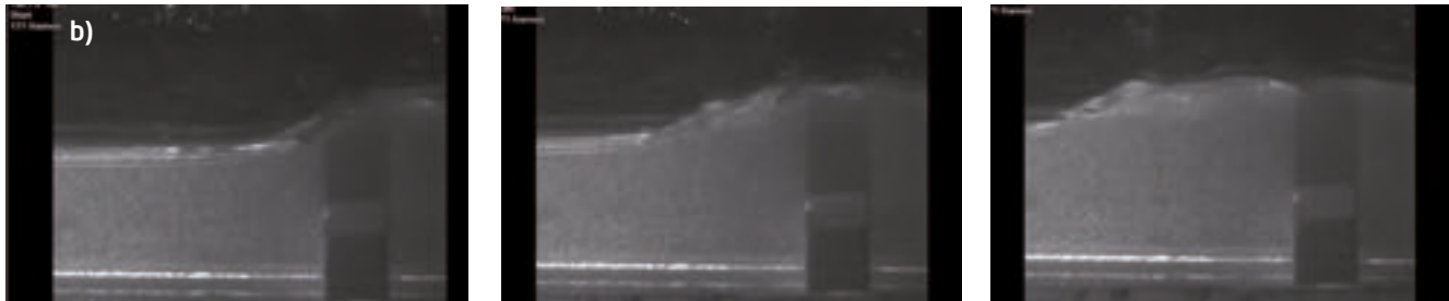
Figure 9: Several images from the experiment showing the sequence of wave propagation. a) At the deep part without barrier; b) Wave breaking due to the presence of the barrier.
